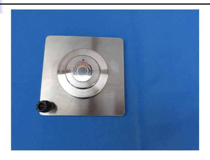
Handling-Procedure Step-by-Step Insert the O-Ring into the cell-body
