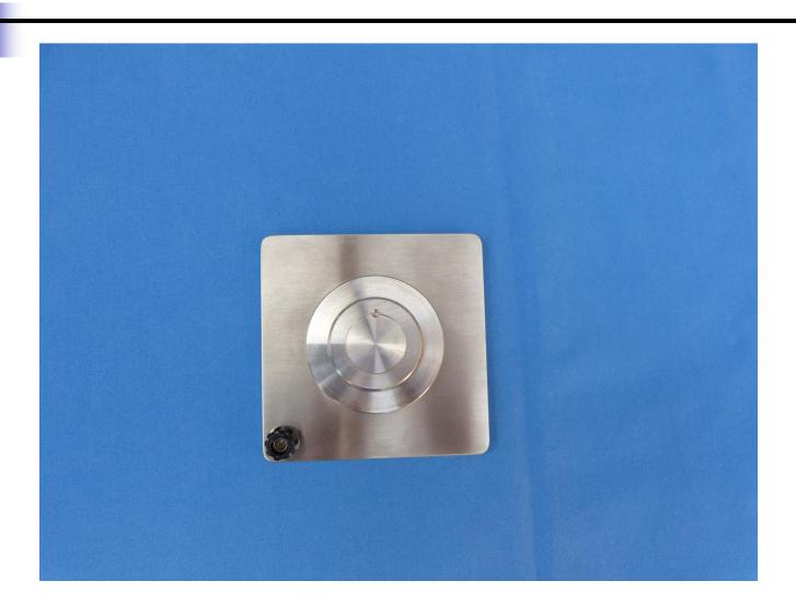
Handling-Procedure Step-by-Step Insert the stainless-steel-planchet
